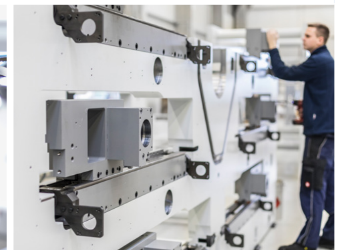
A solid design with 100 mm steel sideframes and outstanding stability as standard
