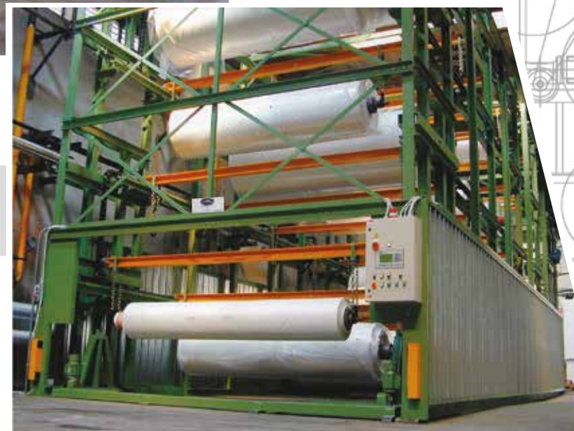
Storaging rolls of fabric by suspending them gives the advantage of avoiding the ovalization given by the crushing occuring when superimposed one on the other
